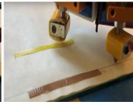
Figure 7: Printing in three modes: T1, M605 S2, and T0, corresponding to Part1, Part 2, and Part 3 in Figure 6 respectively. T0 is the extruder above and T1 is the extruder below.
