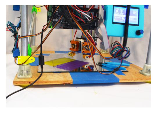
Figure 3: Full layer of the maximally parallel-printed simple diamond shape. With both nozzles printing for the entire shape, we can achieve maximum speedup.
